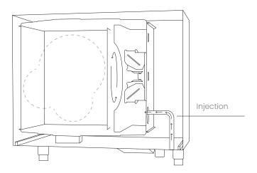
Water is injected in small portions directly onto the heating element and then circulated by the fan to obtain an instant steam generation filling the cavity on all levels.
