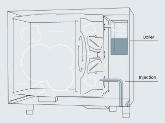
Water is injected directly onto the fan and circulated through the heating element to create an instant steam generation filling the cavity on all levels. Steam is created in the boiler and combined with the injection system, which ensures fast steam production and high-density saturation intelligently controlled by the oven.
